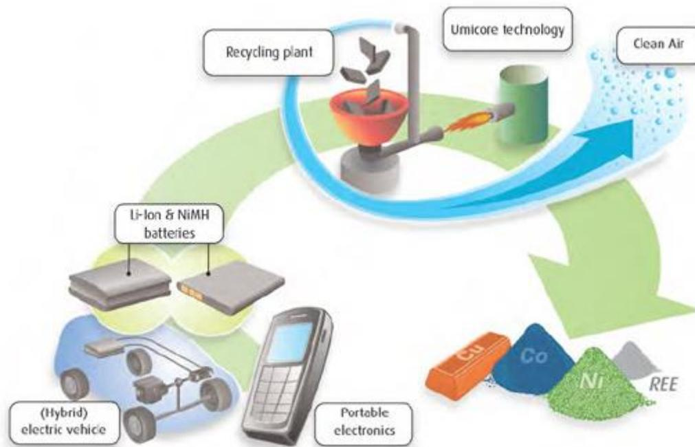
For the new generation of batteries (Li-ion and NiMH batteries), no dedicated process existed. In the best case, they could be rendered inert to avoid the release in nature of hazardous compounds, or to recover some materials, like aluminum and plastics. But most of the valuable compounds – primarily metals like cobalt and nickel – were lost.
